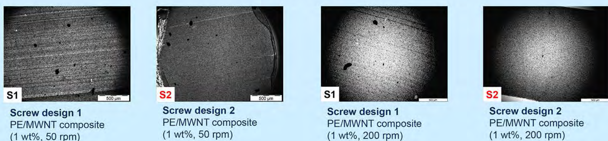
Light microscope images of composites which were compounded with the screw designs 1 and 2 at 50 rpm and 200 rpm
