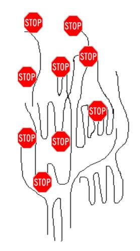
Restricted chain movement (particularly in the amorphous segments) as a result of established chemical and physical bonds between the polymer chain and the nanoparticles.
