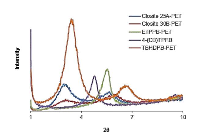
In case of the slurry compounded nanocomposites, higher d-spacing in the TBHDPB-PET composites.
