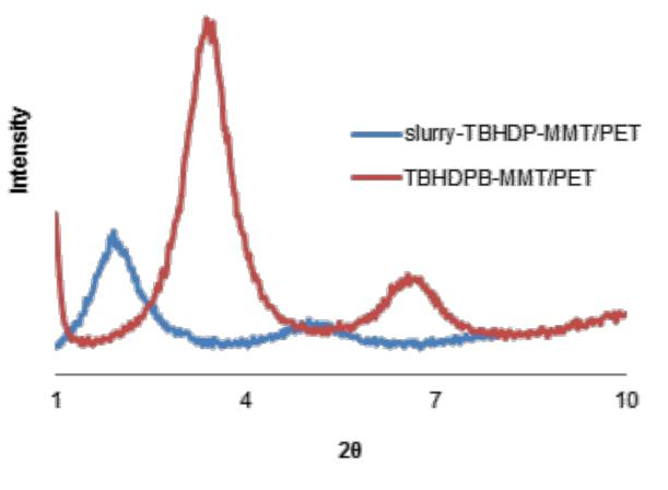
The effect of slurry process can be clearly seen in the d-spacing values as an increase from 2.61 nm to 4.6 nm in the basal spacing.
