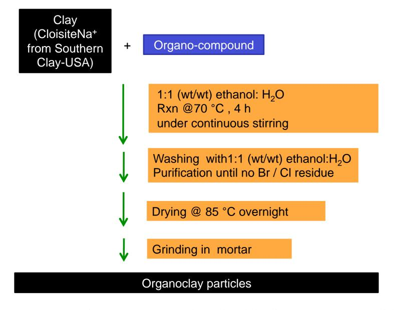
Organoclay particles were mixed with the polymer either in a conventional melt mixing procedure or in a slurry form made with a terpene solvent (Electron<sup>TM</sup>). POSS's were conventioanly mixed with PET.
